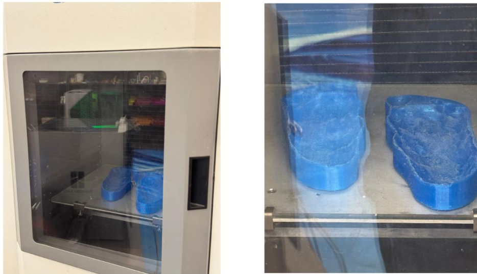
Figure 3: The patient specific footwear being 3D printed in the 3D printer using TPU filament.
