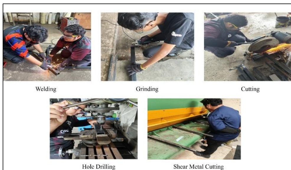
Fig. 8 Fabrication processes of the mechanical components for the ADCS structure
