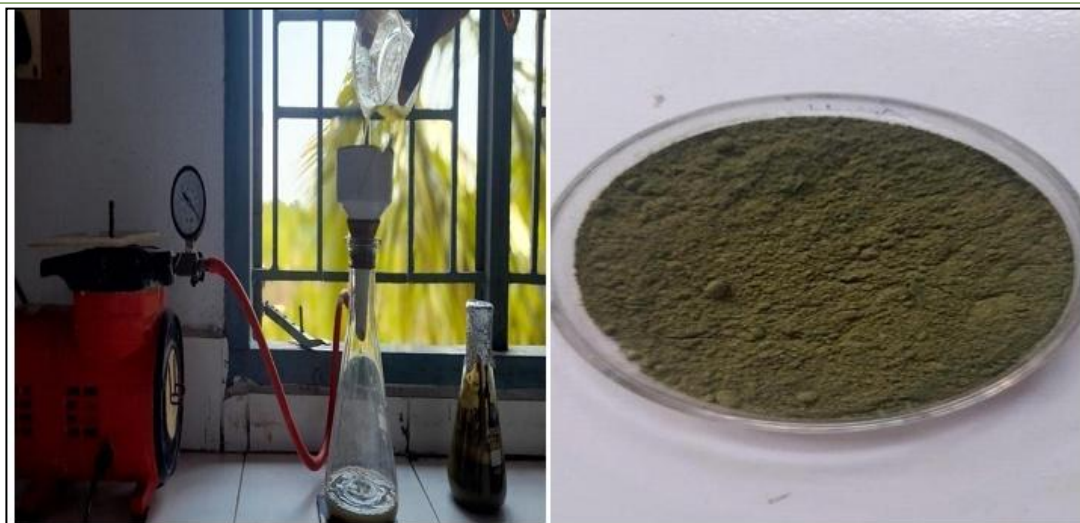
Fig 3: vacuum filtration of extract and grinded powder form of leaves in petridish
