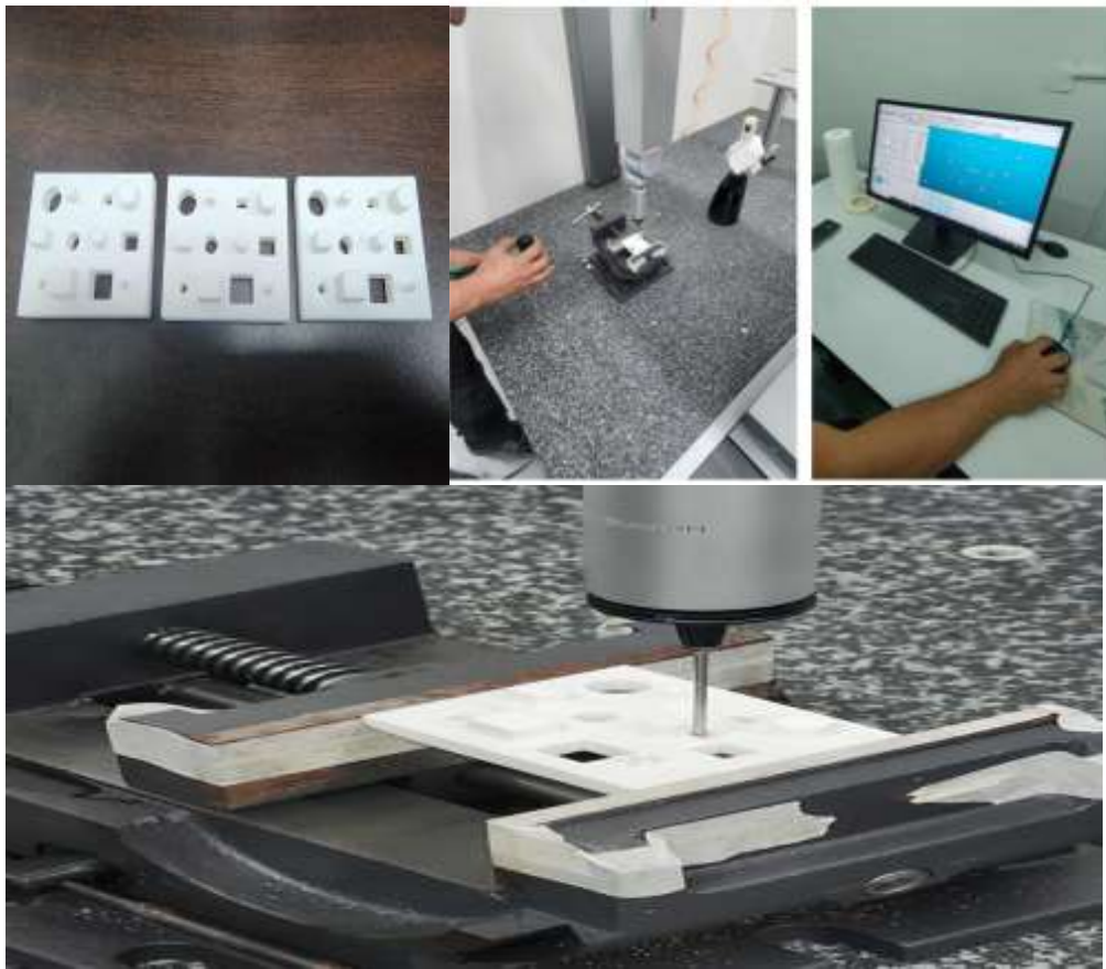
Figure 3. Actual 3D-printed parts and dimensional inspection using a Coordinate Measuring Machine (CMM)
