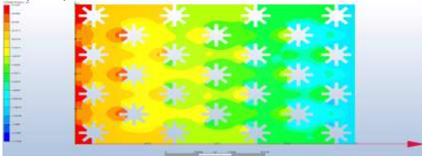
Fig. 15 Static pressure graph in CFD for turbulent flow
