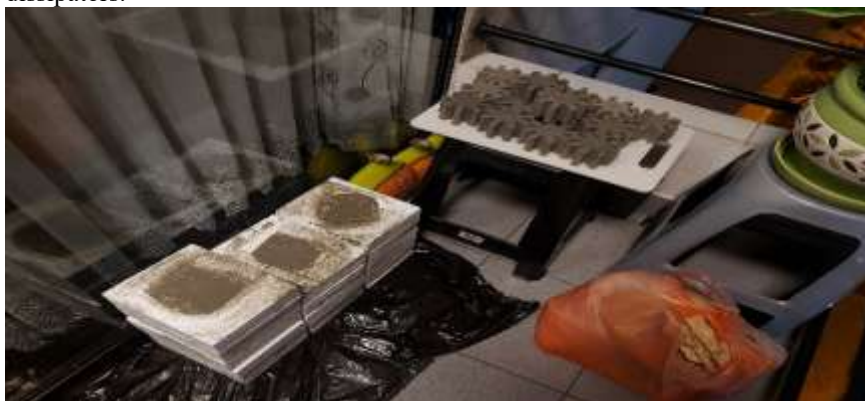
Fig. 5 Molding and de-molding process
