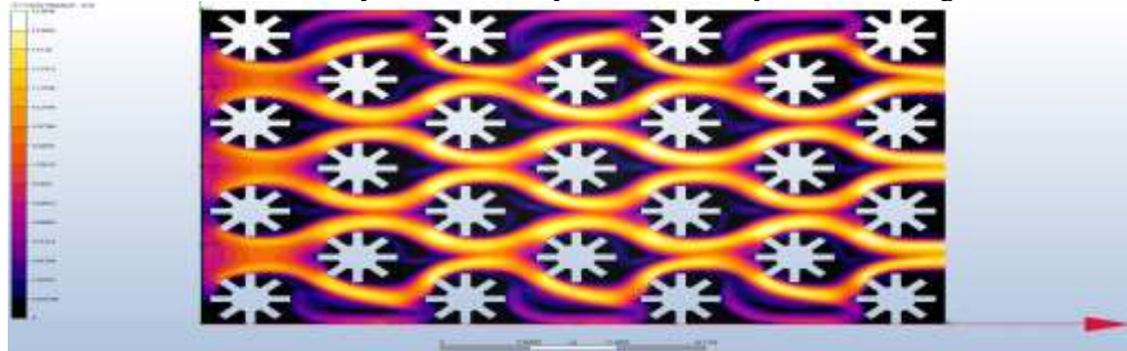
Fig. 8 Laminar flow simulation with a velocity of 0.0101 m/s in Autodesk CFD
