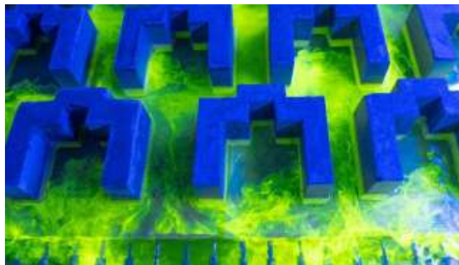
Fig. 15 Generation of longer duration contrails due to negative pressure
