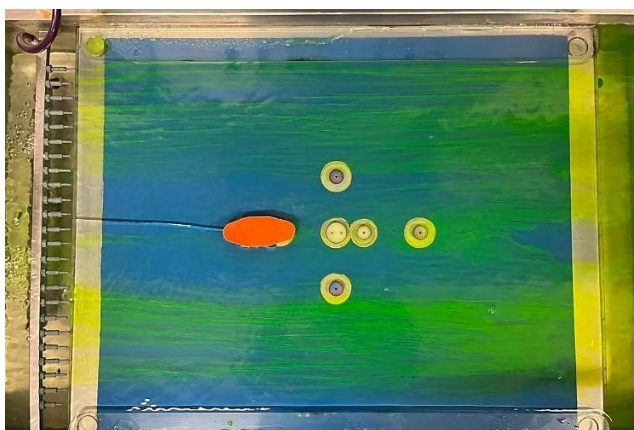
Figure 10 Laboratory photograph of turbulent flow drag in 0^\circ elliptical profile.
