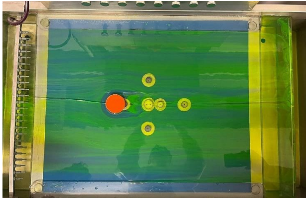
Figure 8 Laboratory photograph of drag with laminar flow on a circular profile.
