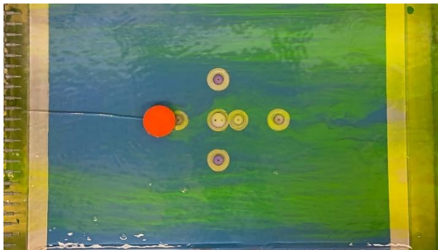
Figure 9 Laboratory photograph of drag with turbulent flow on a circular profile.
