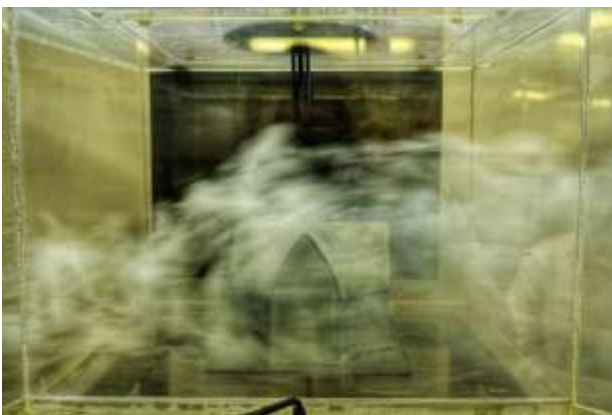
Fig. 20. Profile view of the wind tunnel with a flow velocity of 5m/s.
