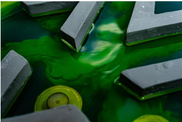
Fig.17 Simulation on the flow table for laminar case.
